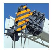
Formed boom made with highyield steel which reduces the operating weight of the boom and maximizes performance.
