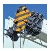
Formed boom made with highyield steel which reduces the operating weight of the boom and maximizes performance.
