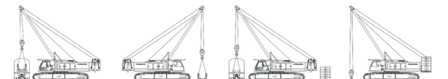
Unloading and assembly of rear counterweight
