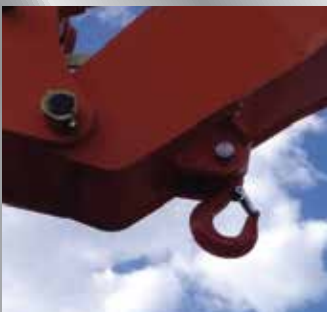
Boom Lift Point
