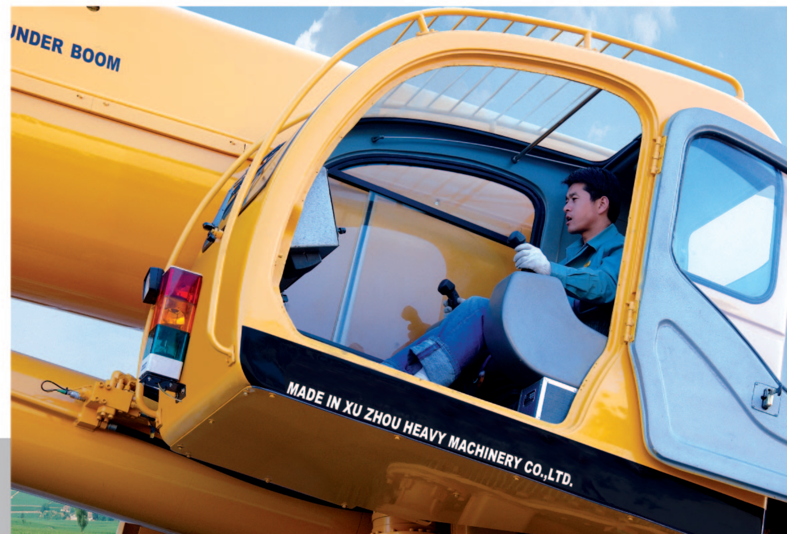
Streamlined upper cabin cab made of compound material can be titled backwards 20°
