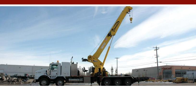
The WHL35TC97 is a natural evolution of our popular 30-ton cranes. Higher lifting capacity and longer reach are obvious benefits of this new design. The versatility of integrated out and down outriggers allows for crane set-up in space restricted areas. These cranes have a wider total spread than other outrigger styles, and a dual control station design means the crane can be operated from either side.
