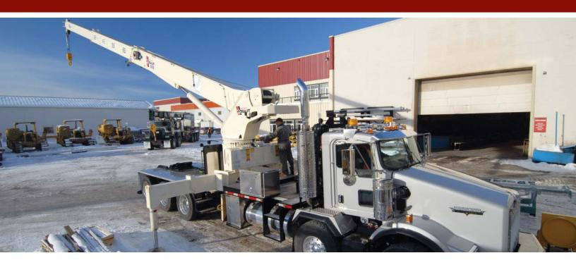
The WHL35TC75 is a natural evolution of our popular 30-ton cranes. Higher lifting capacity and longer reach are obvious benefits of this design. The versatility of integrated out and down outriggers allows for crane set-up in space restricted areas. These cranes have a wider total spread than other outrigger styles and a dual control station design means the crane can be operated from either side.
