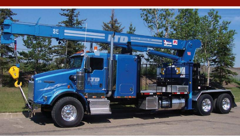
Designed as a mid-range crane, the WHL23TC60 is suitable for multiple applications where a 60 ft reach is required. The design shares the popular hydraulic control console and components with our classic WHL 30-ton cranes.
