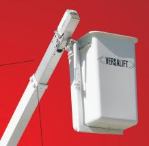
provides 42" insulation gap in fully retracted position available
