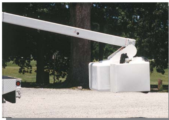
Standard features include hydraulic platform tilt for operator rescue and easy platform clean-out.
