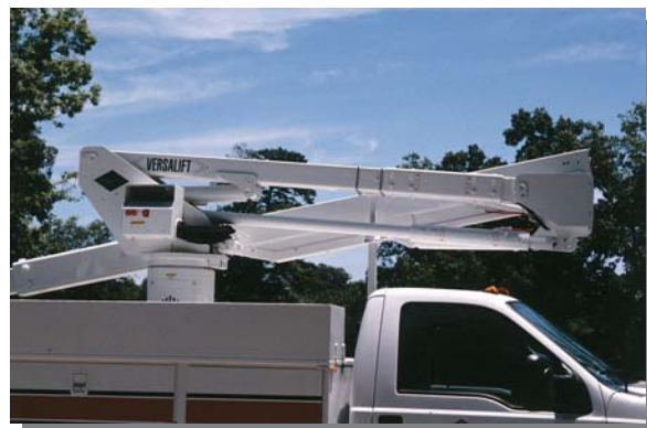
Side by side low stow boom design allows for safer platform entry and reduced travel height.
