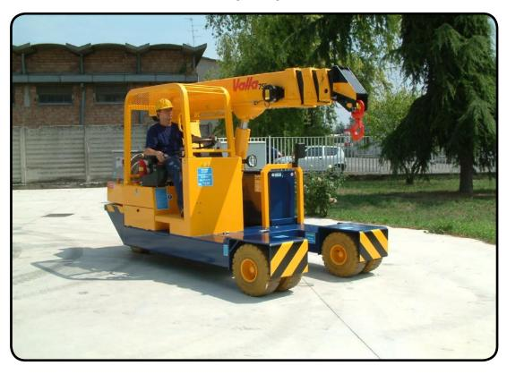
**DRIVE:** DC 8 kW - 48 V fanned, reversible electric motor with MOSFET electronic control HF and energy saving, self diagnostic, speed and temperature checks (no. 2 thermostasts), brush wear warning.
