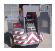
CRANE FRAME: Made by preformed and welded steel plate with built-in counterweight.
