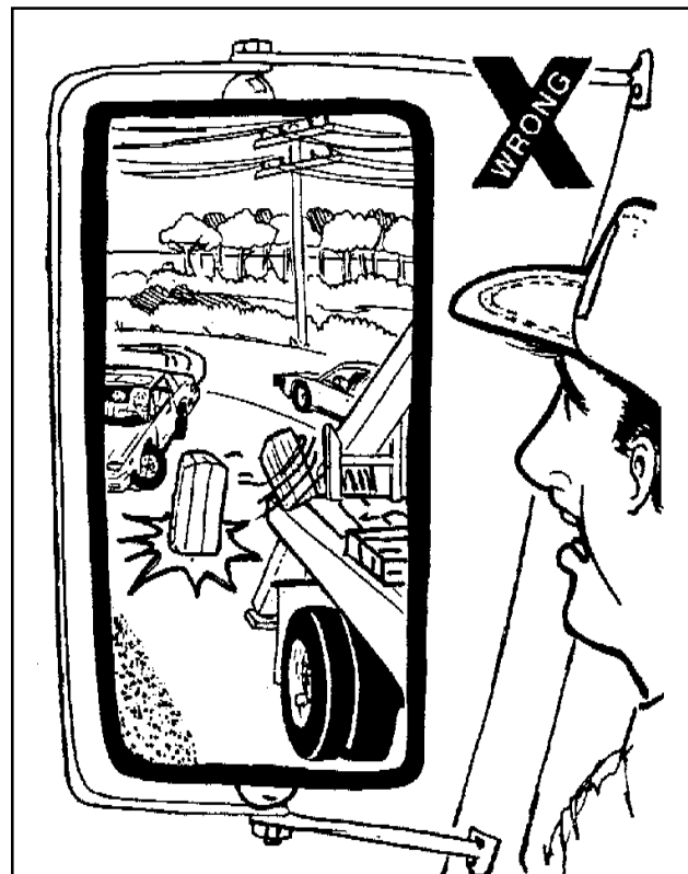
Figure 1-10. Avoid Overhanging Loads
