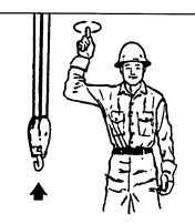
HOIST. With forearm vertical, fore- LOWER. With arm extended downfinger pointing up, move hand in ward, forefinger pointing down, small horizontal circle.
