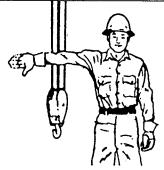
LOAD. With arm extended, thumb pointing down, flex fingers in and out as long as load movement is desired.
