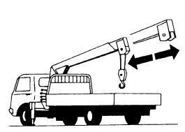
To extend the boom ..... Move the lever to push.
