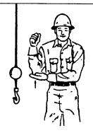
USE WHIPLINE (Auxiliary Hoist). Tap elbow with one hand; then use regular signals.
