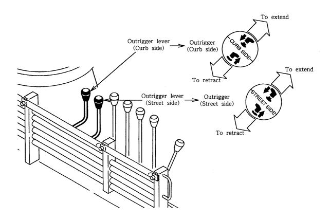
Outriggers: To extend outrigger cylinder, move lever to **push**;
