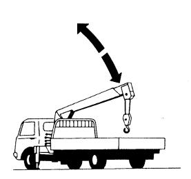
To lower the boom ...... Move the control lever to push.
