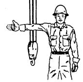
RAISE THE BOOM AND LOWER THE LOWER THE BOOM AND RAISE THE LOAD. With arm extended, thumb pointing up, flex fingers in and out as long as load movement is desired.
