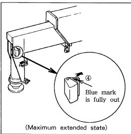
(5) Move the outrigger control lever to push to extend the outrigger cylinders.
