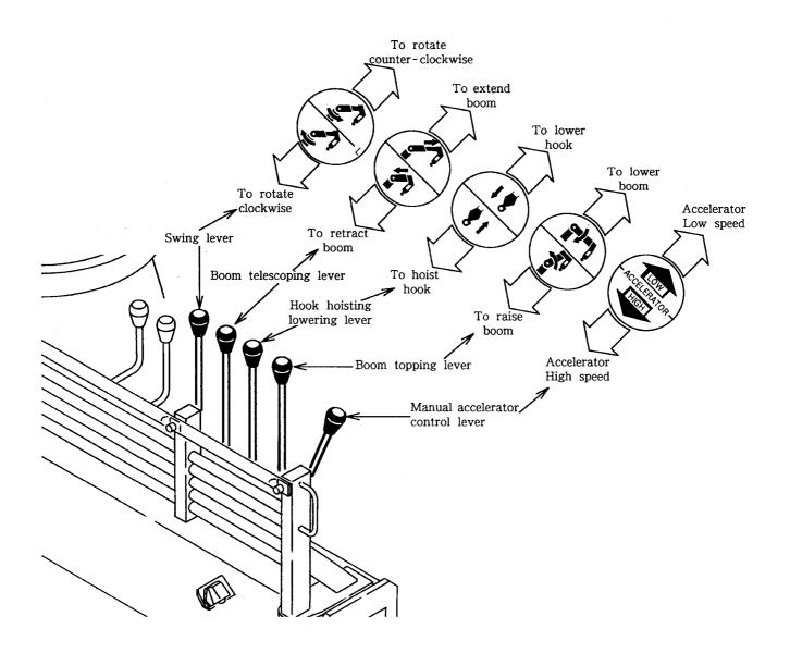
**Boom**: To lower boom, move lever to **push**;
