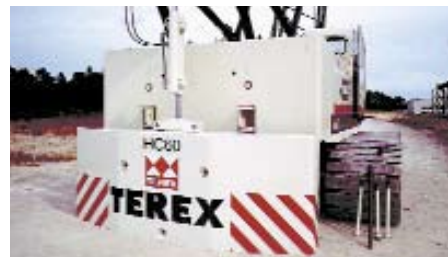
Hydraulic removable counterweight system
