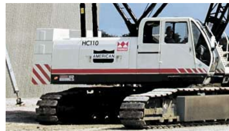
Hydraulic removable counterweight system
