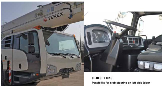
covering) and right side (shift console) of the driver adjustable shift console
