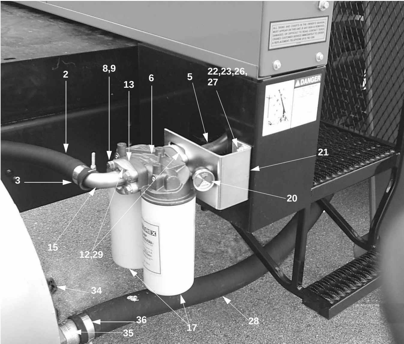
Hydraulic Reservoir & Filter Installation
