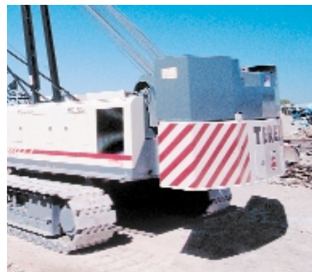
Optional WorkHorse counterweight hydraulically extends for added lift capacity.
