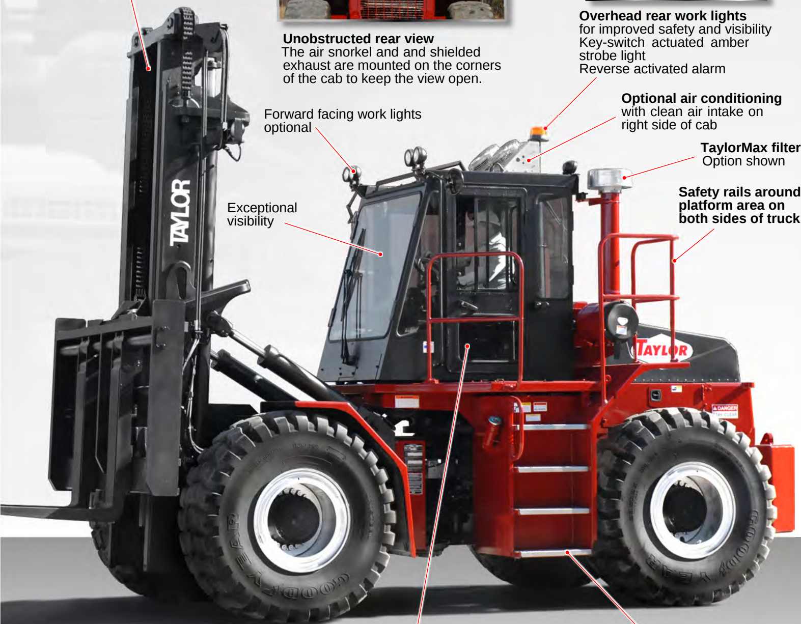
Self cleaning, anti-slip, steps 3-point mounting and dismounting
