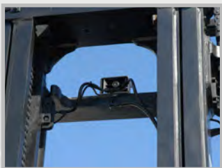
Forward activated alarm
