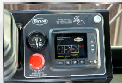
Easy to understand diagnostic display. TICS (Taylor Integrated Control System) using CANbus technology is standard on the TX Series.
