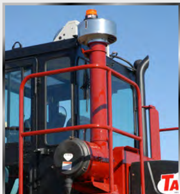
Dual element air cleaner with restriction indicator
