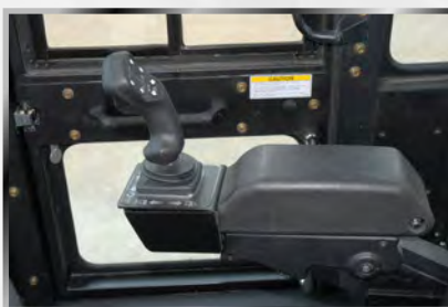
Comfortable adjustable arm rest with fingertip joystick control for smooth precise handling
