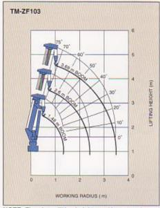
NOTE: The above lifting heights and boom angles are based on a straight (unladen) boom, and allowance should be made for boom deflection
