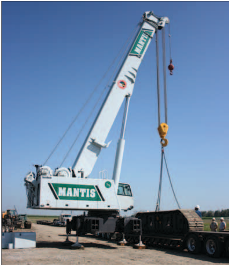
The GTC-1000EX quickly and easily self-erects at job site.
