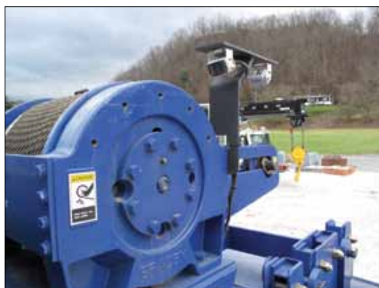
Conveniently positioned cameras display the winch as well as the blind area directly behind the crane. Full color video display in operator cab is standard equipment.
