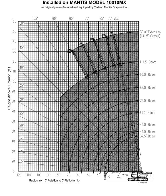
Shaded Area is Allowable Operating Range Limits of operation: Maximum load capacity = 750 lb Maximum radius when mounted on main boom = 78 ft Minimum boom angle when mounted on 30 ft extension = 60°
