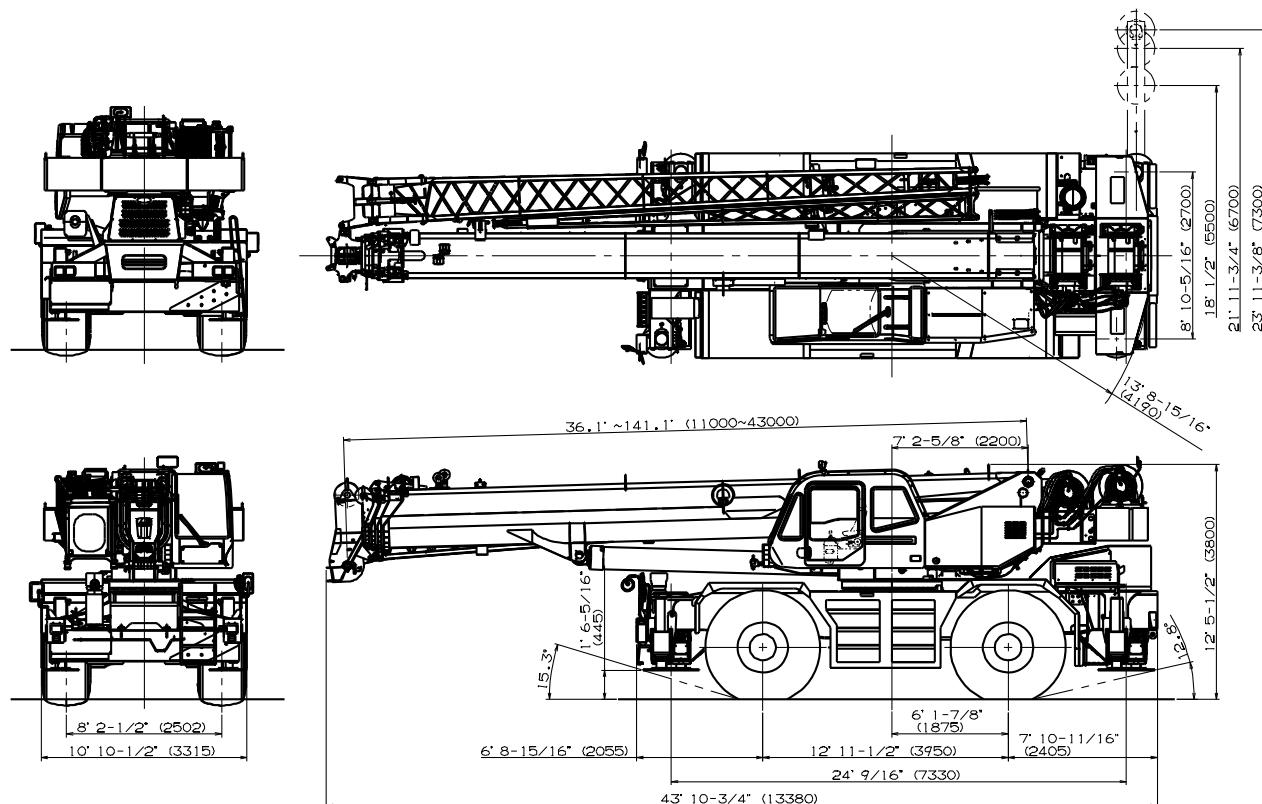
Note : Dimension is with boom angle at -1.6 degree.
