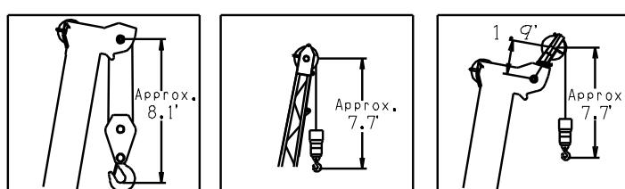
NOTE: 1. Boom and jib geometry shown are for unloaded condition and machine standing level on firm supporting surface.
