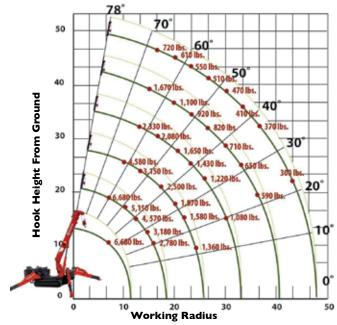
LOAD CHART Lifting capacity varies depending on outrigger configuration and boom length and angle.
