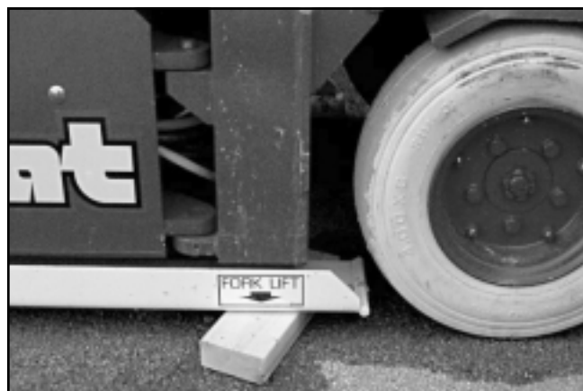
Figure 8.13—Pothole Protector Interlock Test
