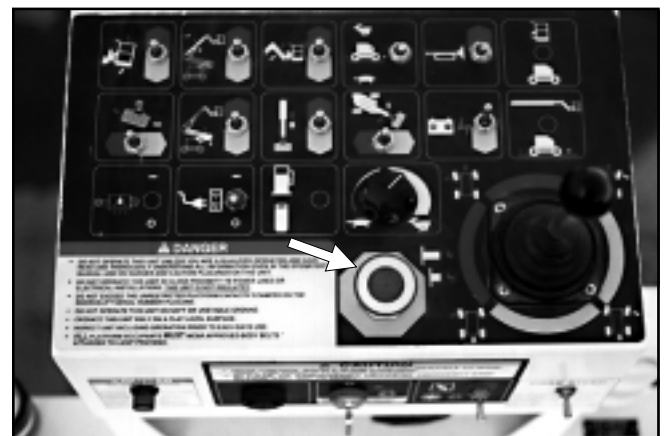
Platform control box Emergency Stop switch location.
