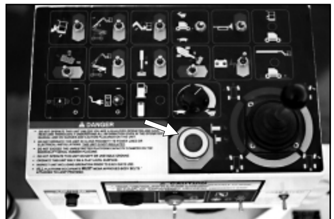
Platform control box Emergency Stop switch location.
