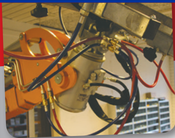
The multifunctional, hydraulic rotary head
