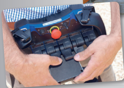
Remote control for all hydraulic functions
