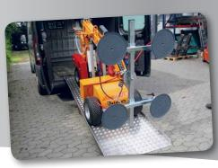
Larger window sections and heavier windows with up to three layers of glass still call for even stronger lifting capacity. SL 608 Outdoor is a new power lift in the Outdoor range and in terms of size it is positioned between the SL 380 Outdoor and the SL 780 Giant
