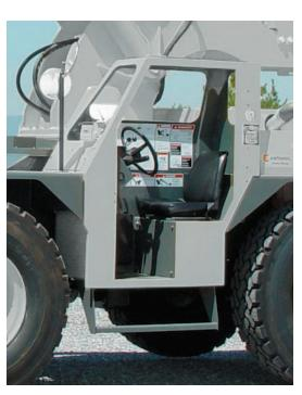
Standard: Open air cab shell w/overhead safety
