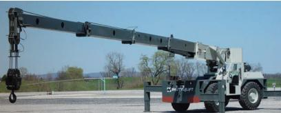
Standard: 4-wheel drive and 4-wheel steer and crab steer with electronic self-
