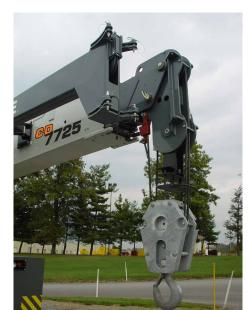
**Hook block** A galvanized coated hook block is provided as standard to help eliminate rusting of this important crane
