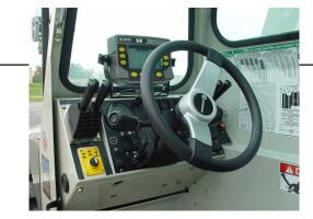
**Operator cab**Hydraulic proportional joystick controls, automotive dash layout, tilt steering wheel, and suspension seat enhances operator comfort and ease of use.
