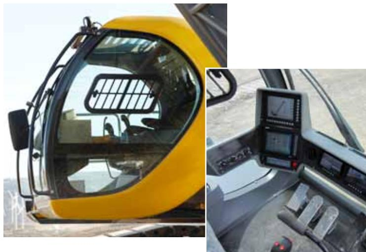
The Ultra Cab, designed by Porsche, maximizes glass space for optimal operator visibility. The working lights and light bar are standard and well positioned. Equipped with adjustable seats and air conditioner. The cab can have a 20° upward angle, and be rotated to the front of platform. Both overhead and bottom view to expand the operating view of drivers and operational safety.
