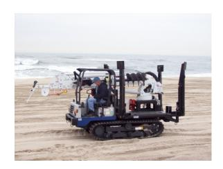
The EZ Track 4100 does not require its full engine power when moving. Set the engine speed relatively low when driving the unit, reserving the higher engine speeds for powering hydraulic accessories.
