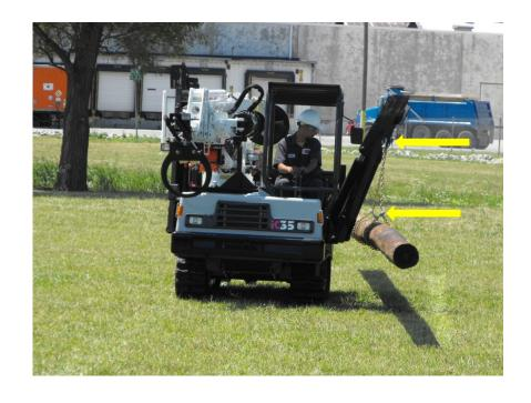
Attach the provided lifting chains to the pole and to the d-rings on the EZ Track 4100 outrigger arms as shown.
