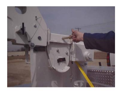
With remote control extend boom to bucket and pin bucket to boom.
