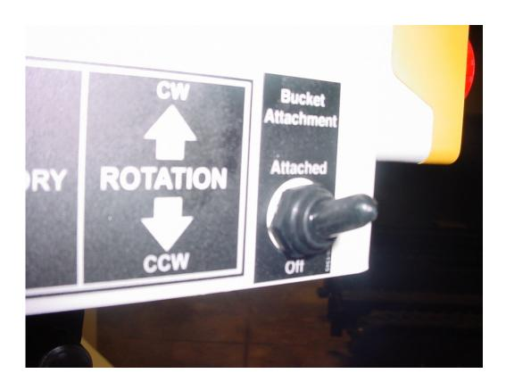
The bucket attachment switch allows for the operator to disable the winch function on the remote control and disengage the H.O.P. overload system as to prevent the operator from locking the unit in a vertical position.
