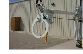
Raise the boom into position so that the lift line will be lifting straight up. Follow load chart specifications on weight in relationship to boom angle.
