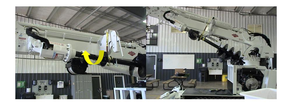
5. Carefully unwind (dig) auger and remove strap. You are now ready to use the remote control to auger as needed.
