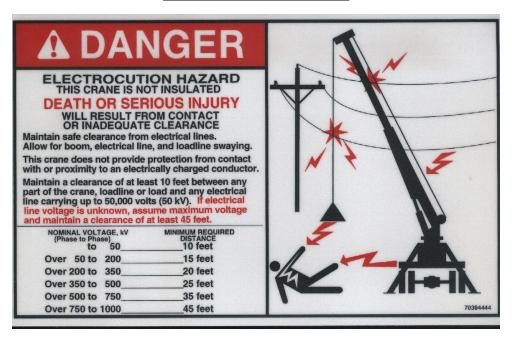
7. Remember even though the the jib is non-conductive, care must be taken to prevent cross fazing. All normal safety procedures must be followed when working with energized lines.
