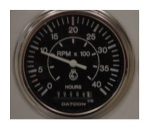
The EZ Hauler 2500 does not require its full engine power when moving. Set the engine speed relatively low when driving the unit, reserving the higher engine speeds for powering hydraulic accessories.
