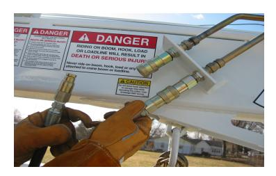
4. Clean the surface of the auger hose and the couplers on the boom. Then attach the auger hose couplers
