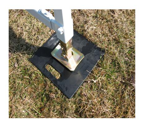
Crank the jack handles to level and support the machine. Oversized outrigger pads might be required depending on soil conditions.
