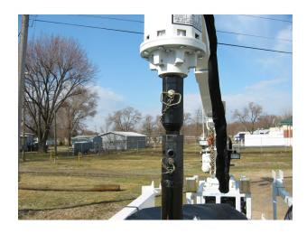
5. Slide extension into auger and pin it in place. Once the extension is in place, align the auger head above it and pin it to the extension.
