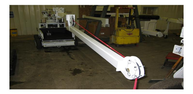
5. Extend the rope out far enough that it can be pinned into the jib sheave assembly. Inspect the rope as you do this, a contaminated rope may cause it to lose its dielectric properties. Now the jib is ready to go to work.
