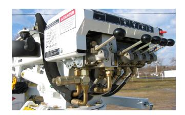
6. Always use the radio remote control to operate the boom. Never use the manual lever override controls to operate the EZ Hauler 2500 because it bypasses the hydraulic pressure overload and can bend the boom sections or tip the machine. These levers are for emergency use only.
