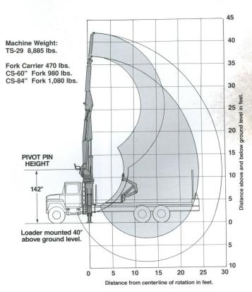
Figures shown here represent maximum hydraulic lifting force available at boom tip for each working radius at various elevations. Figures are maximum possible. Actual lifting capacities will vary with applications and actual worksite conditions. Deduct weight of grapple for payload.
