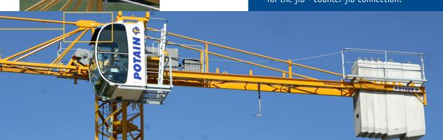
Ballast blocks: 2 types, 3 t and 1 t, allowing different ballasting combinations.
