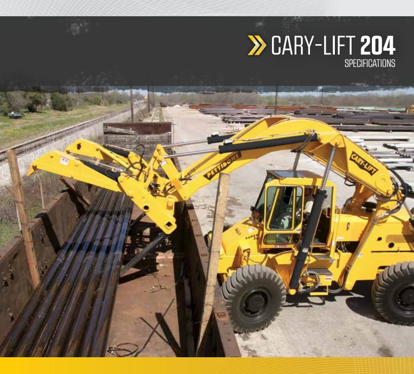
Designed to provide full frontal visibility, the Pettibone Cary-Lift 204 allows operators to lift, place and transport loads with maximum efficiency and safety. A heavy-duty solid steel frame keeps loads stable in full turns. Offering joystick controls and other features for intuitive operation, the 204 provides 90-degree fork tilt down, forward reach, sway control and side shift for unmatched load manipulation.
