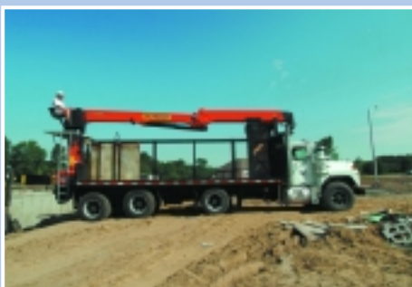
The inline boom stores between the cages
