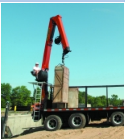
A high inner hook height allows the crane to reach and lift the 1st cage with ease
