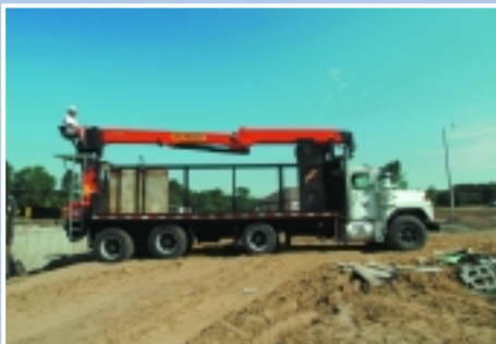
The inline boom stores between the cages
