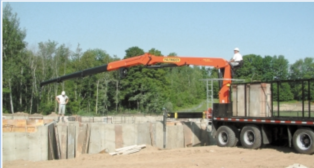
PowerLink™ linkage system gives the outer boom added strength in flat-out position and a constant folding speed.
