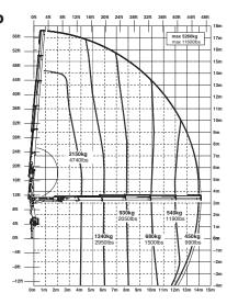
The outreaches stated are with a boom angle of 20° and are therefore not the maximum.
