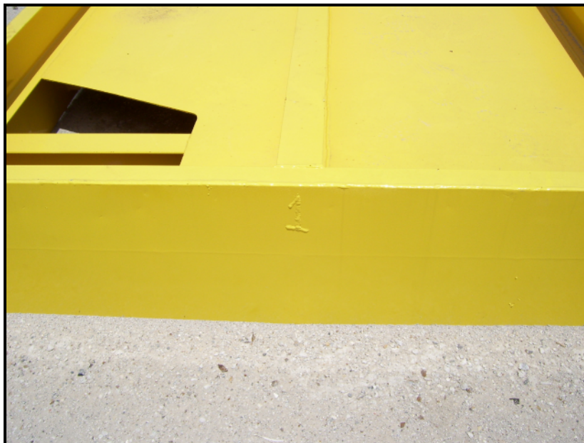
Figure 16 - Mud Mat Marking
