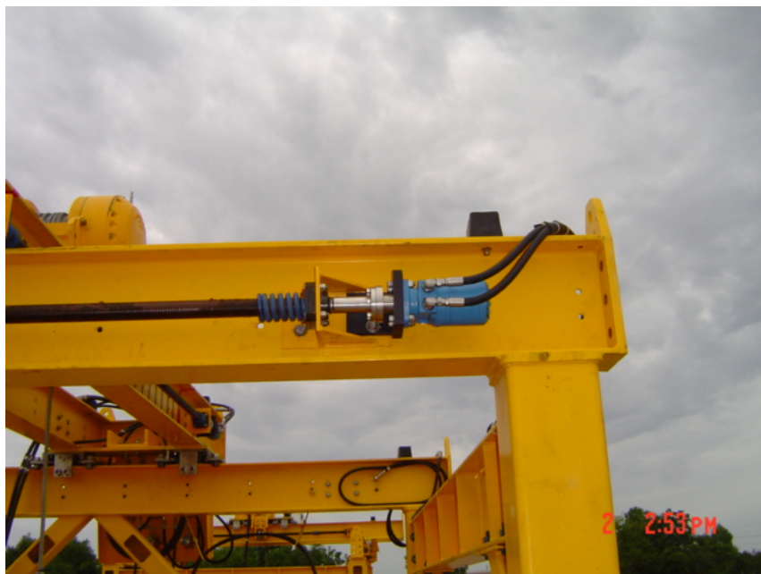
Figure 9 - Acme Drive Hydraulic Motor
