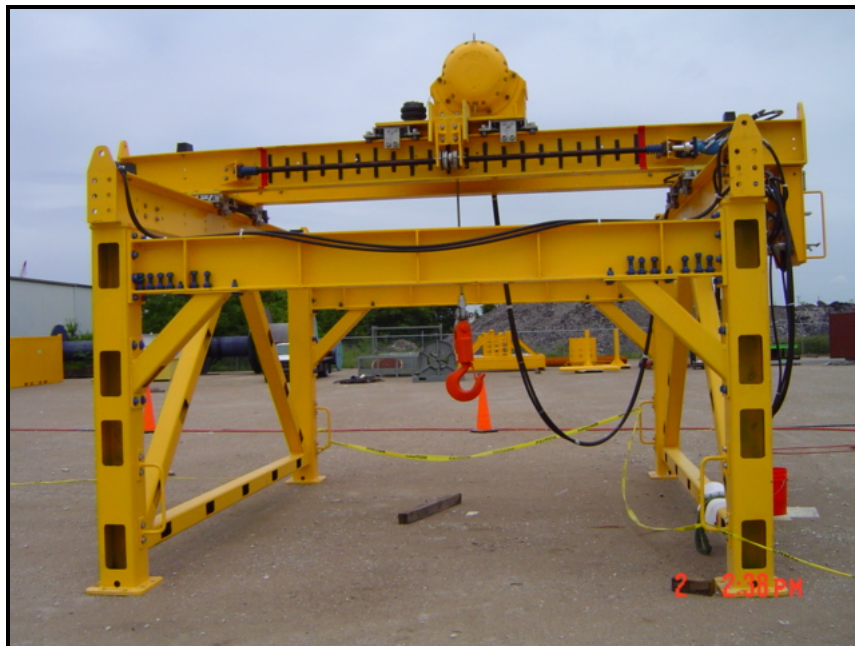
Figure 3 - Gantry Frame (Extensions Removed)
