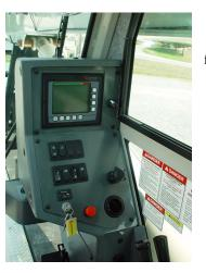
(LMI) is standard on all NBT45 machines. The LCD display is visible in full or low light and displays all crane load lifting values simultaneously. Includes Work Area Definition System (WADS).
