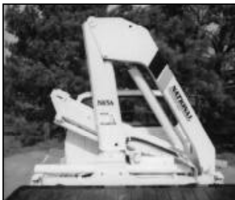
Rack and Pinion Rotation
