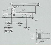
The configurations are based on the Series 600D with an 85% stability factor. The complete unit must be installed in accordance with factory requirements and a test performed to determine actual stability and counterweight requirements since individual truck chassis vary.
