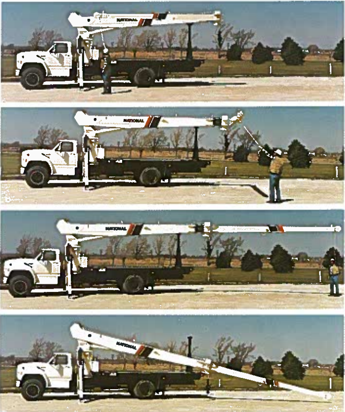
The sequence of photos above shows how a National jib folds into working position.
