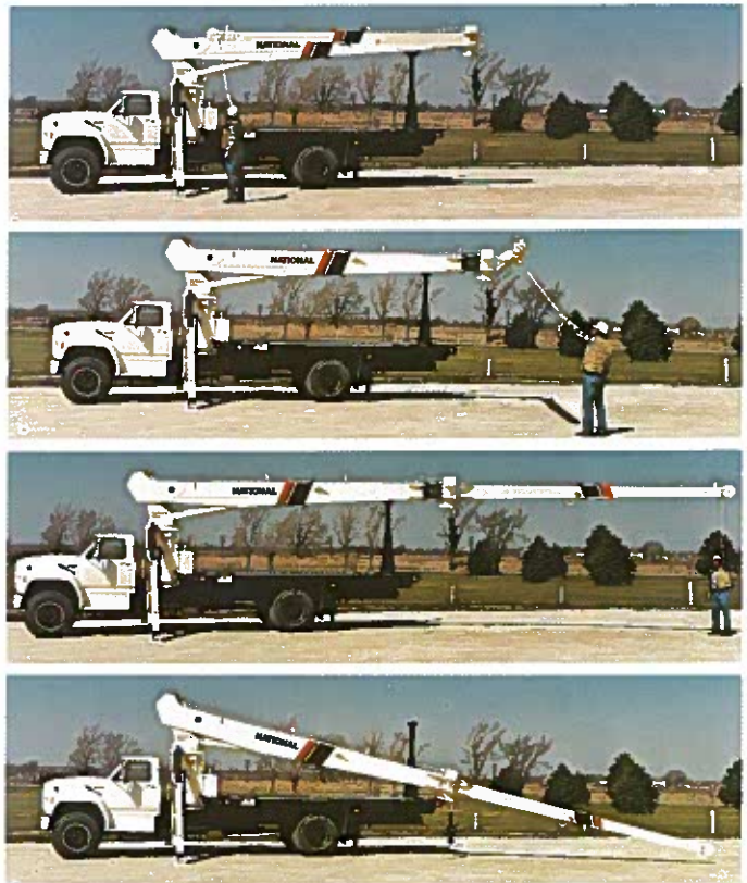
The sequence of photos above shows how a National jib folds into working position.
